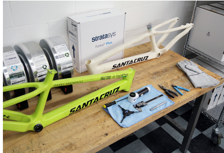
Design concept bike frames 3D printed using ASA material.
