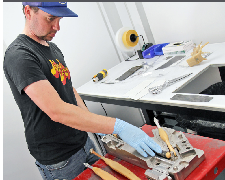
Test fitting a 3D printed ULTEM™ 1010 resin mandrel in the composite lay-up tool used to make the carbon fiber bike frame.
