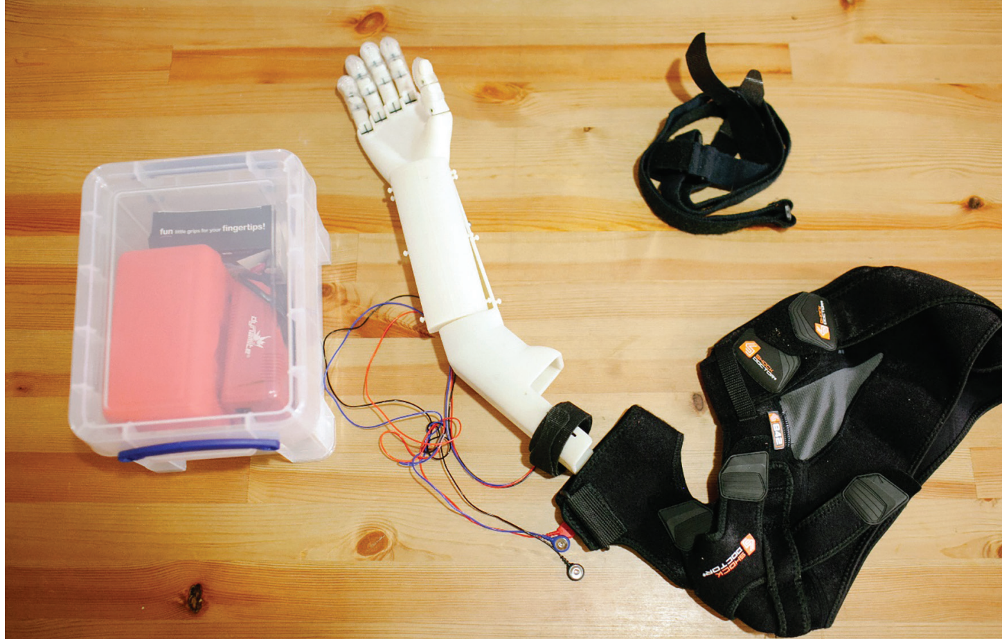
The 3D printed replacement limb is strapped to a neoprene shoulder brace to distribute the arm's weight across Alex's torso.
