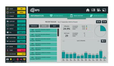
Titanium features a range of reporting tools and dashboards to help users capture build history, parameter detail, hardware usage and part traceability data.
