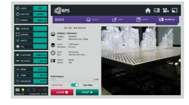
Each NEO system is installed with a built in camera, offering users the potential to keep track of builds remotely, at any stage.
