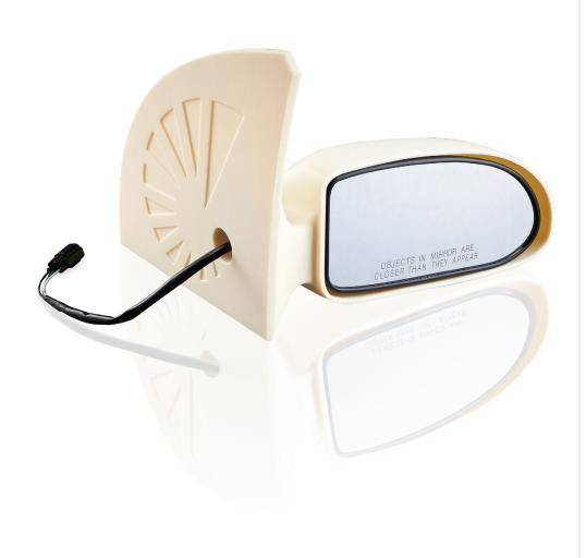
Offering a variety of production-grade thermoplastics, FDM® technology creates parts that are highly accurate, tough and suitable for both functional prototyping and end-use parts. ABS is the most common material used as it boasts good mechanical properties and high name recognition. Compared with ASA, ABS may be more familiar because of its popularity in mass production.
