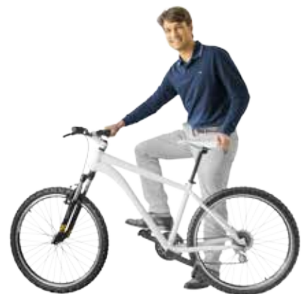
Bicycle frame 3D printed on the Objet1000 and assembled into a fully-functioning bicycle
